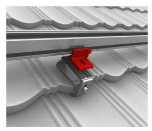
The mounting rail is mounted on the roof hook with the help of of the K2 Climber and the Allen bolt with underhead serration. Tightening torque 16 Nm. Due to thermal expansion, the Rows can be separated after max. 17.6 m. The minimum distance for separation between two K2 rails is 3 - 5 cm. Minor unevenness is compensated by one or more
