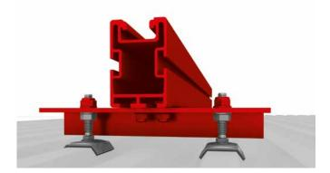
The K2 Bridge is mounted on two solar fasteners instead of the adapter plate in order to achieve greater span widths. Depending on type, the rail is fixed to the Bridge with one or two M10x30 T-bolts.
