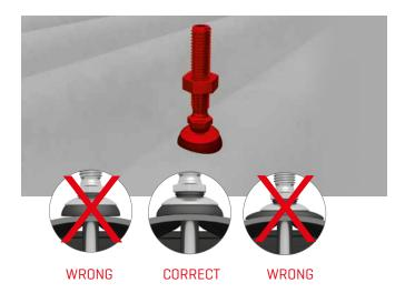
Additional information: Do not tighten the solar fastener with the torque, the seal must be slightly compressed and rest on the entire surface. Materials required: Solar fastener
