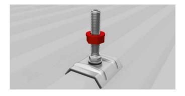
Adjust nut in height according to direction of the module carrier rails. Materials required: Hex nut, washer
