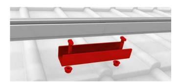
Lay Mounting Rail on joint with rail connector and connect with T bolts and self-locking nuts. The rail joint may not be in the range of the roof fastener. Tightening torgue 16 Nm.
