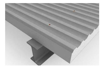
Measure the screw distances according to statics or K2 Base. Check position of purlins and pre-drill through the profile sheets into the purlins.
