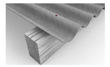
Measure the screw distances according to statics or K2 Base. Check position of purlins and pre-drill through the fibre cement profiles into the purlins.
