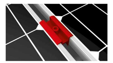
Use two universal module middle clamp OneMid between two modules. Klick the Stance in the notches. Place clamps on the module frames and fix them. Tightening torque 16 Nm.
