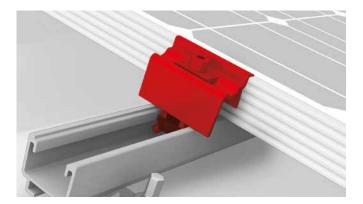
Fix the module in place at the end of a row with universal module end clamp OneEnd. Klick the Stance in the notches. Alternatively use the standard end clamp. Insert the MK2 nut into the mounting rail and turn clockwise by 90°. Place clamps on the module frames and fix them. Never mount module end clamps directly on the rail joint or end of the rail! (Spacing: min. 50 mm from edge of module frame). Pay attention to the mounting instructions by module manufacturer!
